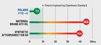
ASTM D8335. In 3rd party testing against 9 competitive products Polaris PS-4 had less than half the deposits compared to the next closest product. No other tested products met Polaris Engineering standards for deposit cleanliness. Test measures mass of deposits in mg in high temp, high stress test cycles. Higher deposits will impact engine power and performance.
